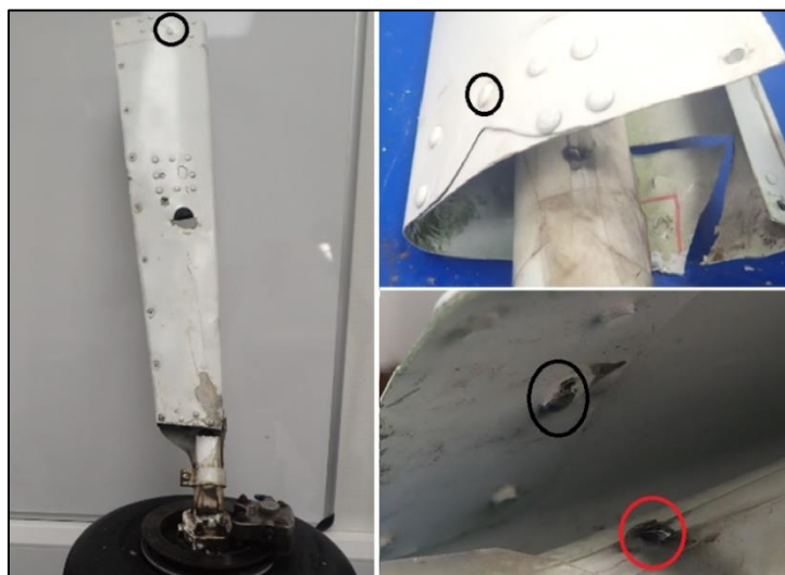
Photo No. 7: Sheet-metal repair & associated damage to undercarriage leg
