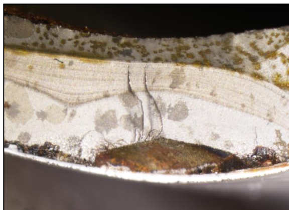
Photo No. 5: Microscopic examination of fracture surface (Wheel side)
