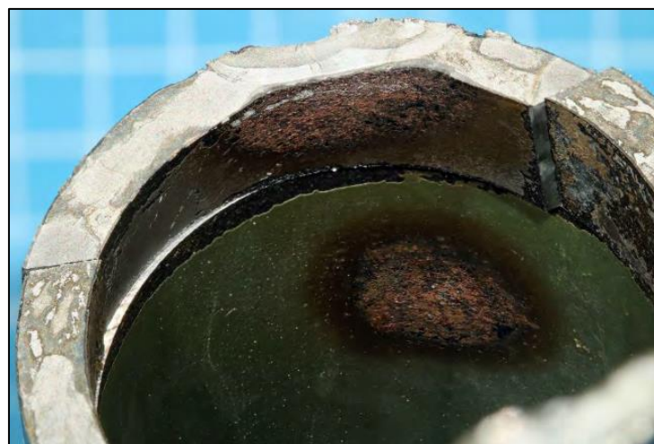
Photo No. 6: Internal heat discolouration
